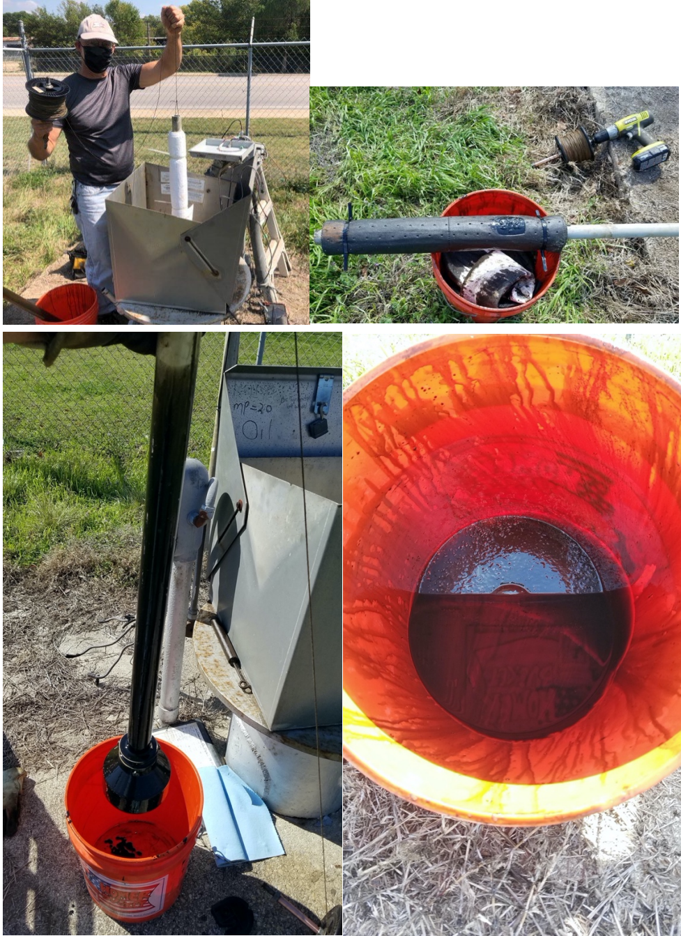
Figure 30 to 33, clockwise from upper right, showing absorbent pads after and before deployment in the well, modified bailer coated in dark oil; and oil water mixture recovered from the well.
