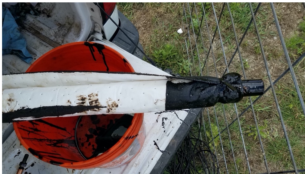
Figure 6. Absorbent pad after deployment in Burnet 5809303. Only the bottom eight inches of the pad made contact with the oil layer.
