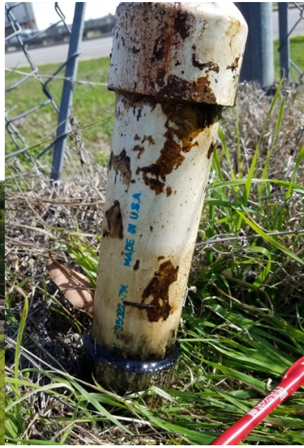
Figure 16. Float from the Karnes well showing a coating of clear oil on the PVC.
