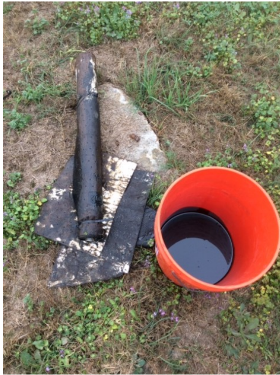
Figure 17 (left). Used pads and recovered oil.
