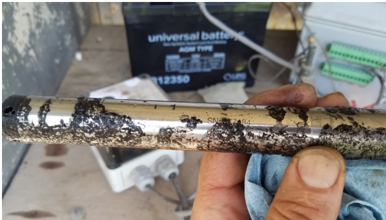
Figure 19. Tarry material on the transducer from the Milam recorder well.
