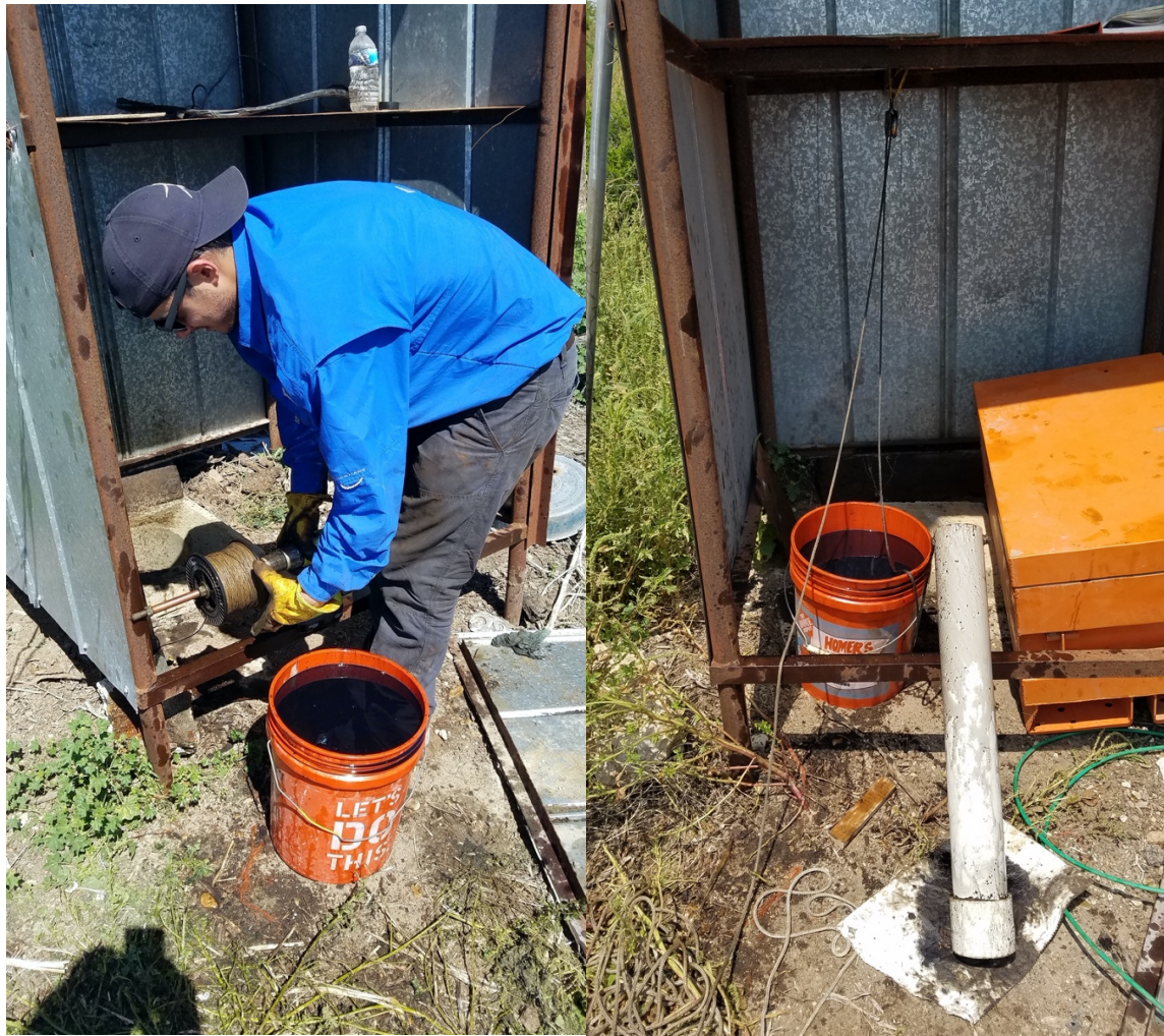
Figures 37 (left) and 38 (right). Oil recovered on 5/5/21 using product-only bailer and oil recovered on 7/7/21 using 3-inch bailer.
