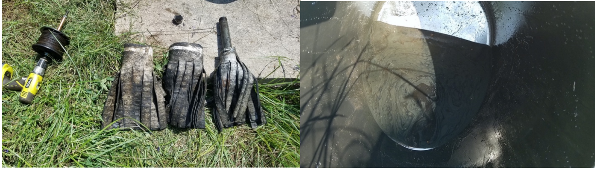
Figure 34 and 35. Absorbent pads cut into mop configuration (left) and oil film on water recovered after oil removal (right).
