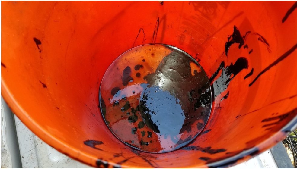
Figure 7. Oil and water recovered from Burnet 5809303, showing high viscosity of recovered oil.
