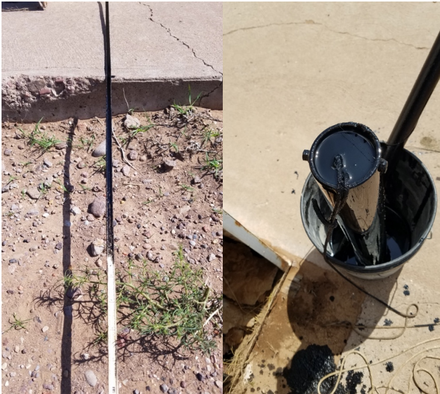
Figure 23 (left). Dark oil on the interface meter tape.
