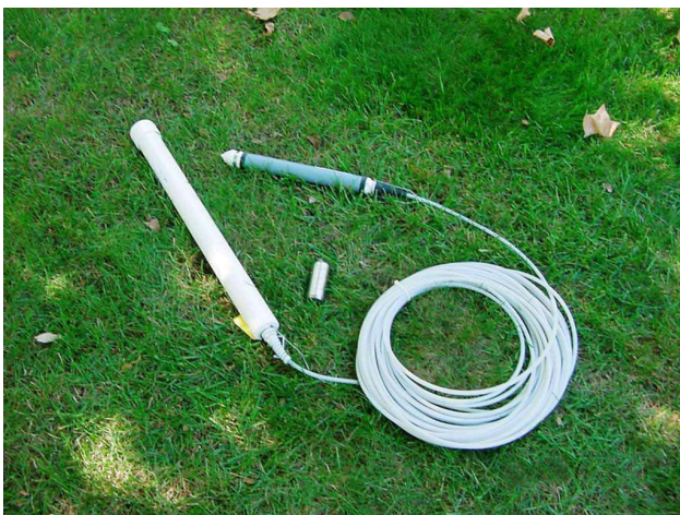
Pressure transducer used for continuous water-level monitoring.
