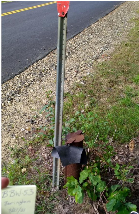
Figure 1. Photos of the protective surface casing of BBW-53 before (left) and after (right) replacement of the surface protective casing.
