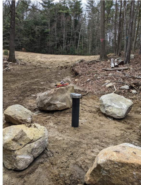
Figure 2. Protective surface casings for replacement overburden well LMW-36 (left) in Litchfield, NH and NGWMN expansion well KEWB-01 (right) in Keene, NH,
