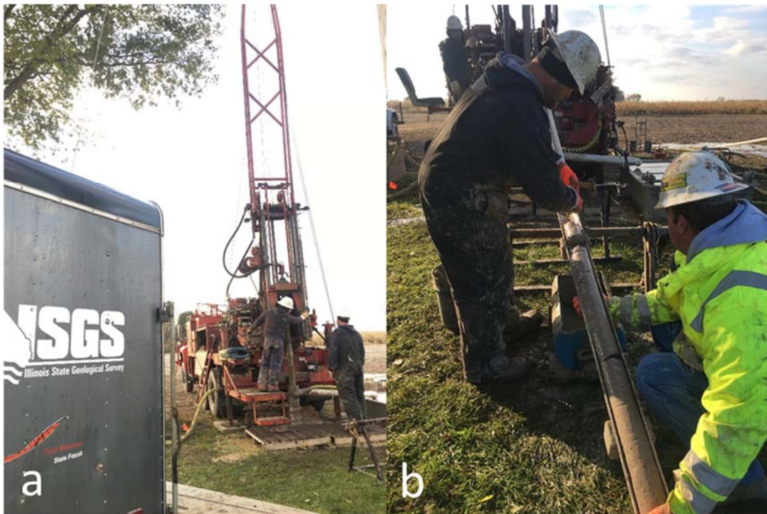
Figure 2. (a) Rear view of CME drilling rig operated by the ISGS and (b) extraction of continuous core from the wireline sampler.
