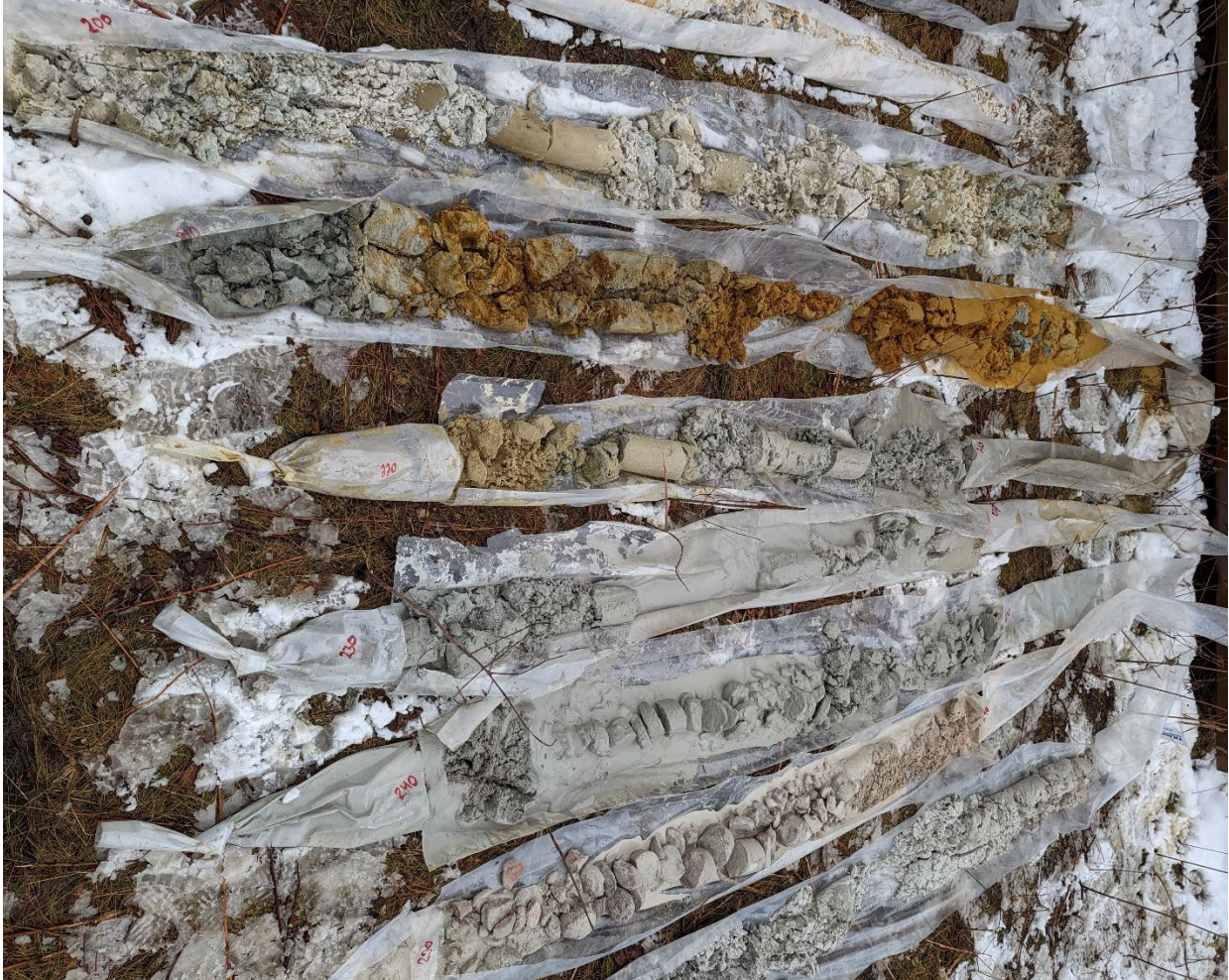
Figure 2: Continuous drill cores recovered using the roto-sonic drill method. Note the footages are labeled on the bags; the 200ft to 210ft interval is at the top of the photo, and 250ft to 260ft interval is near the bottom.
