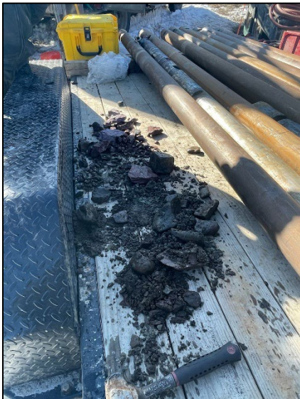
Figure 13. Sand, gravel and cobbles were blown from the well.
