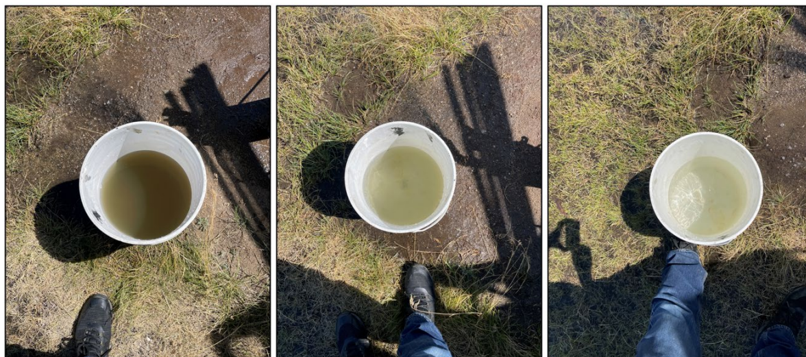
Figure 18. MBMG-4719. The well was pumped until the discharge cleared.
