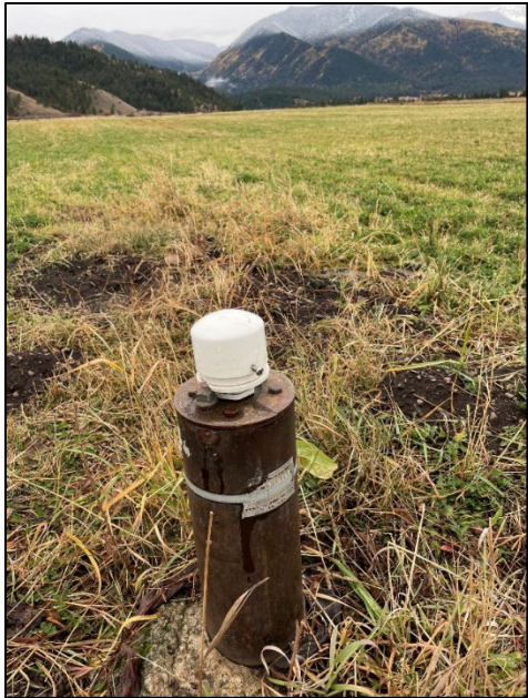
Figure 6. MBMG-76048. The well is only accessible through a small measuring port; well has a GPS location.
