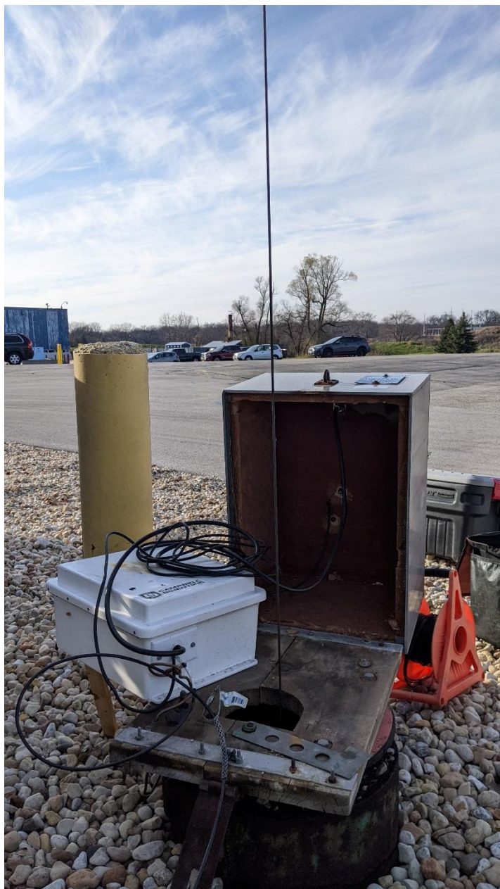
FIGURE A4. CLOSEUP (LEFT) AND WIDER (RIGHT) VIEW OF THE WIRELINE LOG ACQUIRING DATA AT FERMILAB WELL #2 AT SITE 1.
