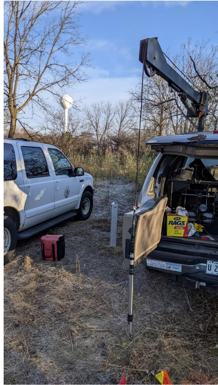
FIGURE A11. THE WELL WITH THE ACOUSTIC TELEVIEWER PROBE (LEFT) AND THE WATER LEVEL METER AND FLUID TEMPERATURE AND RESISTIVITY PROBE (RIGHT)
