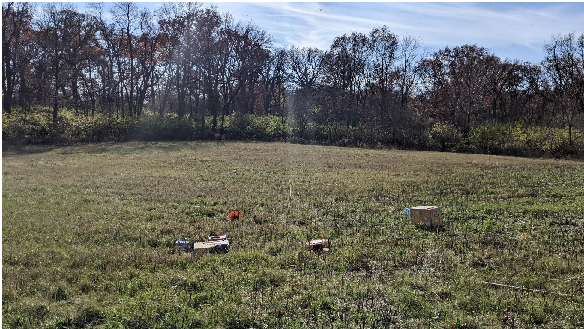
FIGURE A7. WALKTEM SETUP AT SITE 2. BARELY VISIBLE IS RED TRANSMISSION LOOP EXTENDING TO RIGHT AND LEFT FROM ORANGE REEL.
