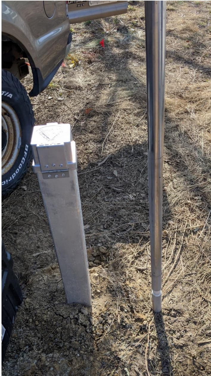
FIGURE A11. THE WELL WITH THE ACOUSTIC TELEVIEWER PROBE (LEFT) AND THE WATER LEVEL METER AND FLUID TEMPERATURE AND RESISTIVITY PROBE (RIGHT)
