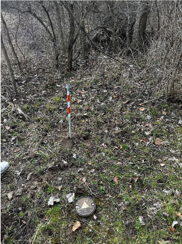
Figure 5. Photograph of the reflective post added at Rushville_S site next to the flush-mount well.
