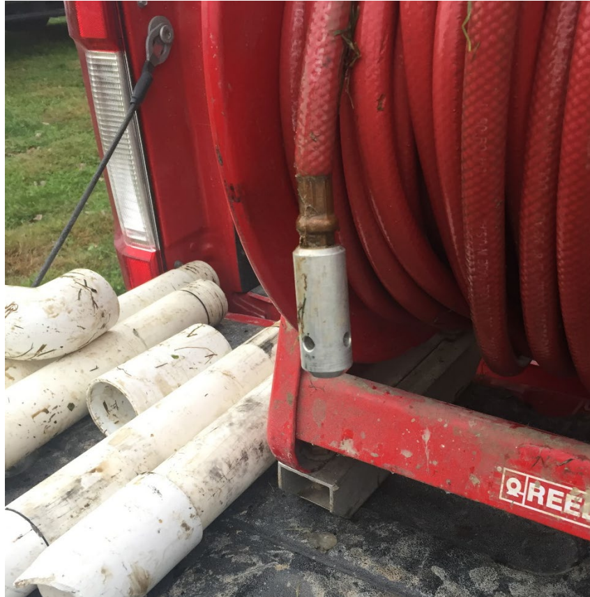
Figure 6. Photograph showing specially constructed nozzle at the end of the compressed air line that directed compressed air at 90 degrees into the well screen slots to aid well development.
