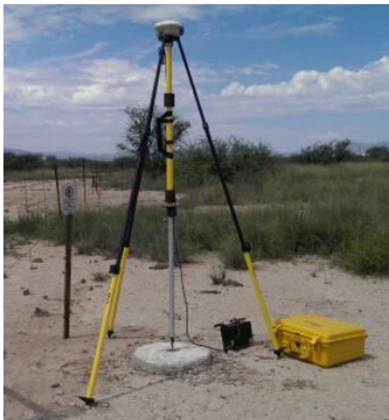
Typical GNSS Survey Setup
