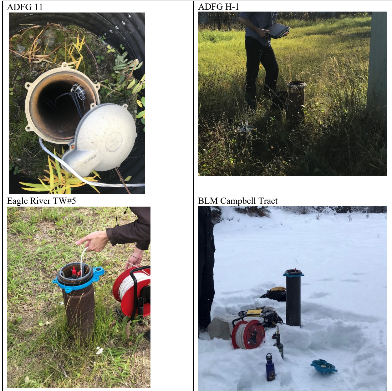
Fig 4. Location photos of monitoring wells ADFG-11 and ADFG H-1 at former ADFG hatchery within the Fort Richardson military base. The recently rehabilitated and re-instrumented monitoring well in Eagle River (lower left), and the newly drilled well at the BLM Campbell Tract (lower right) in the Anchorage Bowl.
