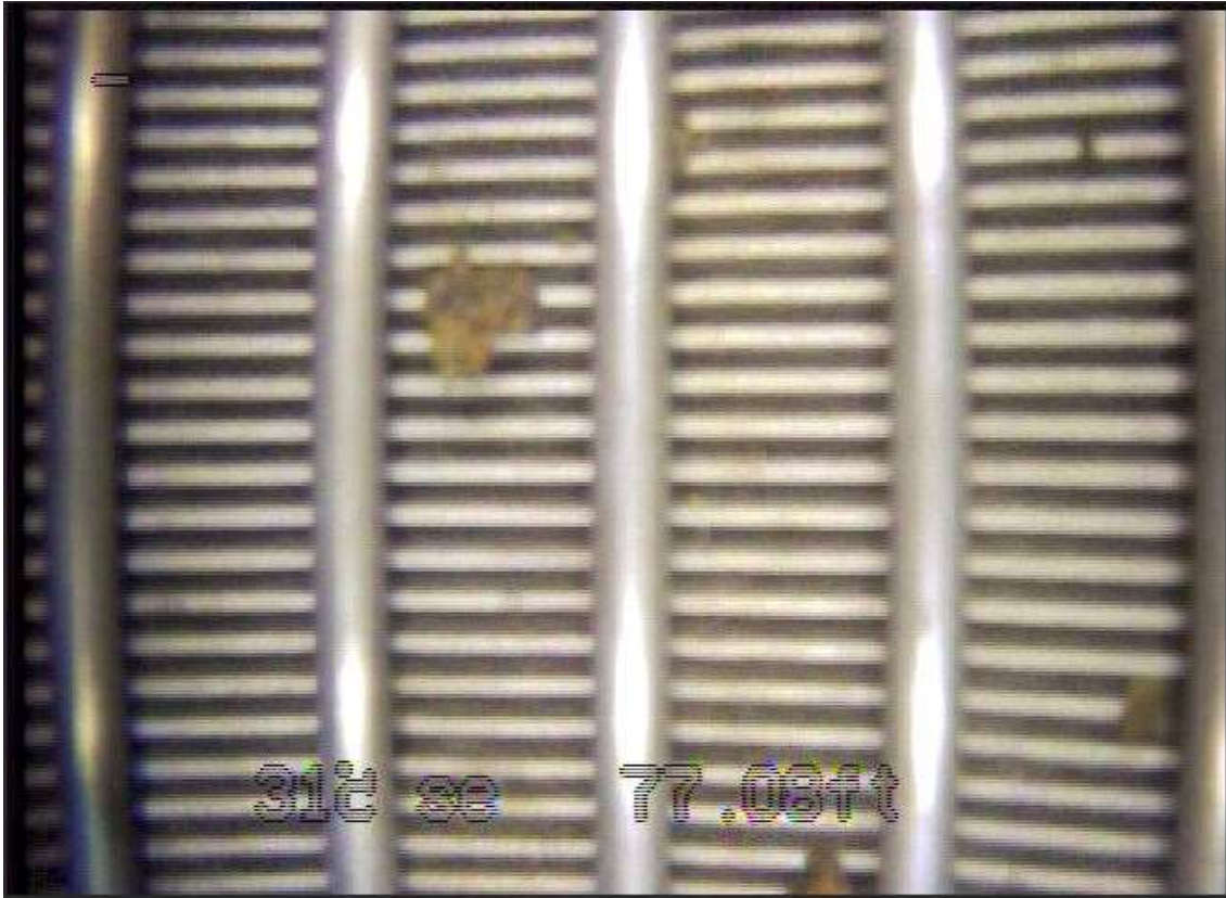
Figure 5. Lateral view of screens in well MTG-6, GSAL111889, Montgomery County, Alabama, at 77.08 feet as shown by down-hole camera survey. Note orange scale material from casing above attached to unobstructed screen. Image from down-hole camera video survey collected by a Strahl Borehole Dual Inspection camera on May 10, 2022.
