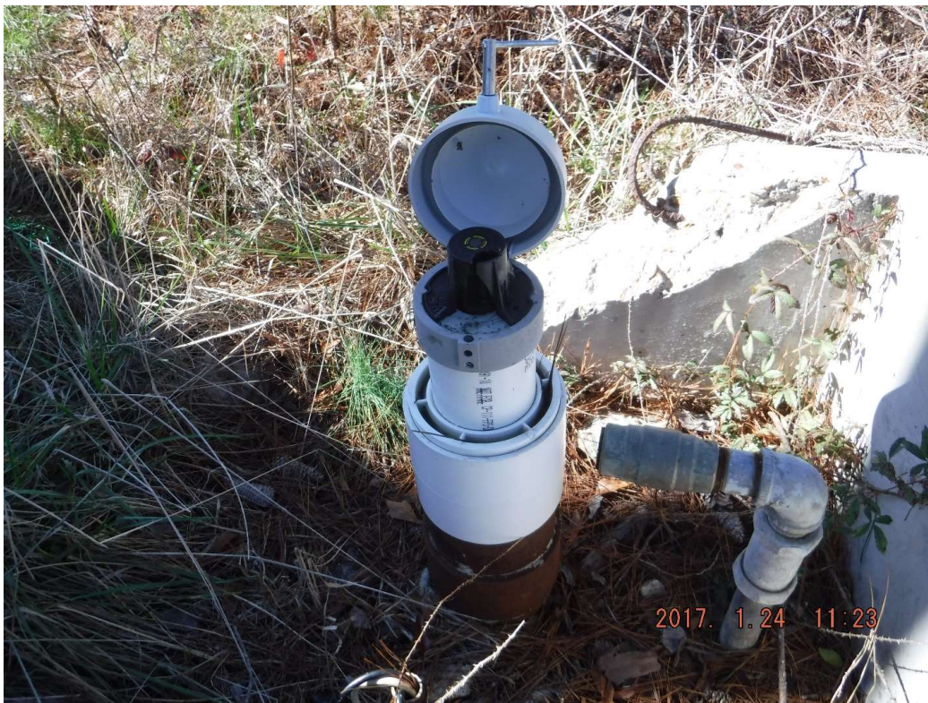
Figure 3.—Geological Survey of Alabama well MTG-6, GSAL111889, Montgomery County, Alabama. Image highlights OTT EcoLog 1000 pressure transducer, data logger, and locking collar and cap installed on the well casing.
